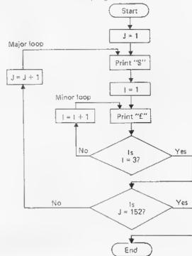
You can jump <u>out</u> of a loop at any time. If you do this the loop control variable will remain at whatever value if had got to when you jumped out. In our case the loop control variables were J for the major loop and I for the minor loop.
