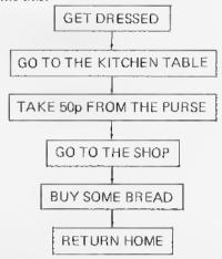
Each box contains an instruction, and the arrows show the order in which the instructions are executed. Well, that looks pretty simple and neat. Now that the flow diagram is drawn on paper we can check it by going through the boxes one by one and asking ourselves: Can the child (or the computer) do this?
