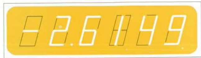
Fig. 3. Displayed characters are generated by modulating these figures. The digit 1 is shifted to the center of the pattern.
