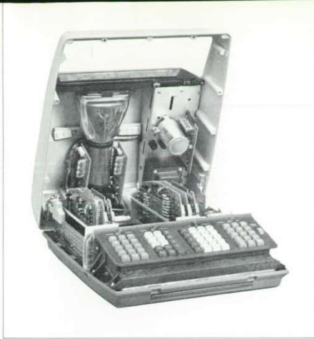
Fig. 5. Internal adjustments of the calculator are easily accessible by removing a few screws and lifting the top.
