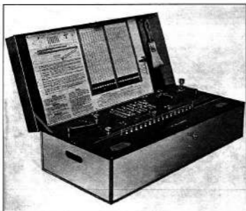
FIG. 1. MILLIONAIRE CALCULATING MACHINE WITH 16 PLACES IN THE PRODUCT
